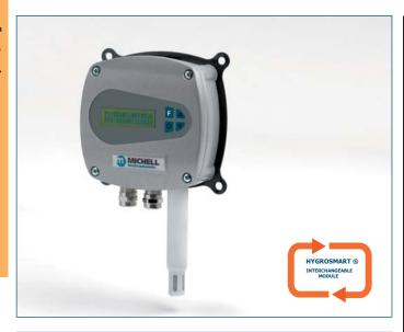
The WM291 relative humidity transmitter includes the interchangeable Hygrosmart module. The interchangeable module lets you recalibrate the transmitter simply by replacing the sensor head with the Hygrosmart module. As a result, maintenance costs are greatly reduced and down-time is minimized.
