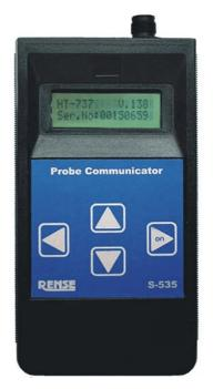
The S-535 is a versatile digital handheld meter which is designed for the new  $\mu$ Controller based humidity and temperature sensors from Rense Instruments. It is capable of displaying the data of humidity probes as well as programming and calibrating them. This gives the user the possibility to change the probes parameters and settings especially when in the field.
