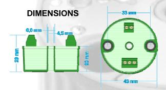
**Super saver!** A reliable low-cost analogue transmitter to convert a Pt100 (RTD) 3-wire input signal to 4-20mA. Select the range you want by just making a solder link on top of the transmitter, and fine adjusted by a multi-turn potentiometer.
